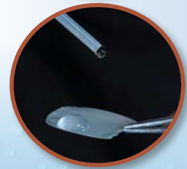
Wolfgang Sigmund demonstrates how water drops retain their shape on the almost frictionless surface his team developed, instead of bulging out as they do on an untreated surface in the lower inset.
