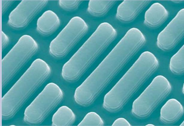
*UF materials engineers have tapped elements of sharks' unique scales to develop an environmentally friendly coating for ship hulls that prevents the growth of algae and may also impede barnacles. The coating is composed of billions of tiny raised diamond-shaped patterns, each measuring about 15 millionths of a meter.*
