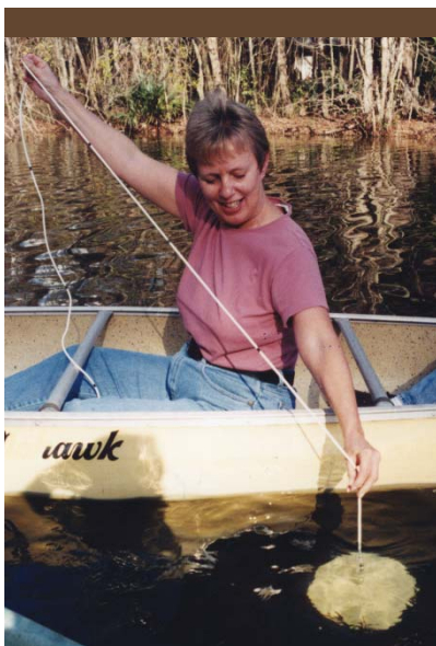
Phyllis Brumfield uses a Secchi disk to determine water clarity on Clear Lake. Volunteers lower the disk into the water until they can no longer see it and then record the depth. The more algae in a lake, the faster the Secchi disk disappears.
