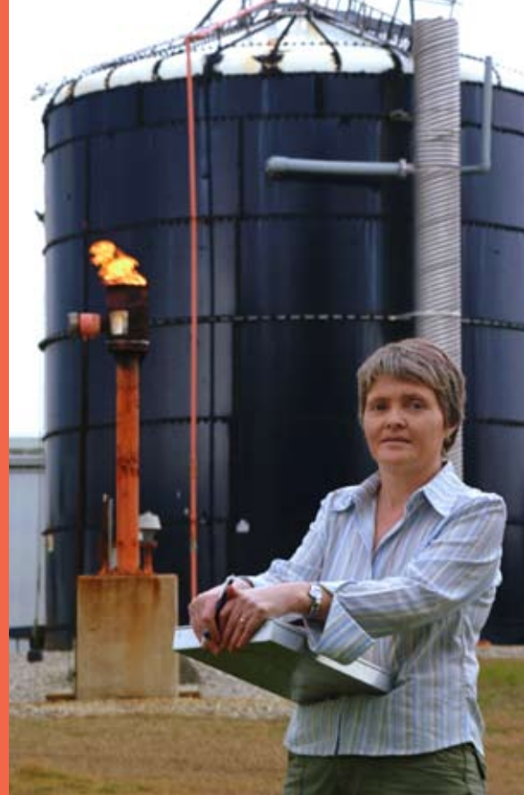
Ann Wilkie records data at the waste treatment system at UF's Dairy Research Unit in Hague. The fixed-film anaerobic digester tank produces methane gas from flushed manure
