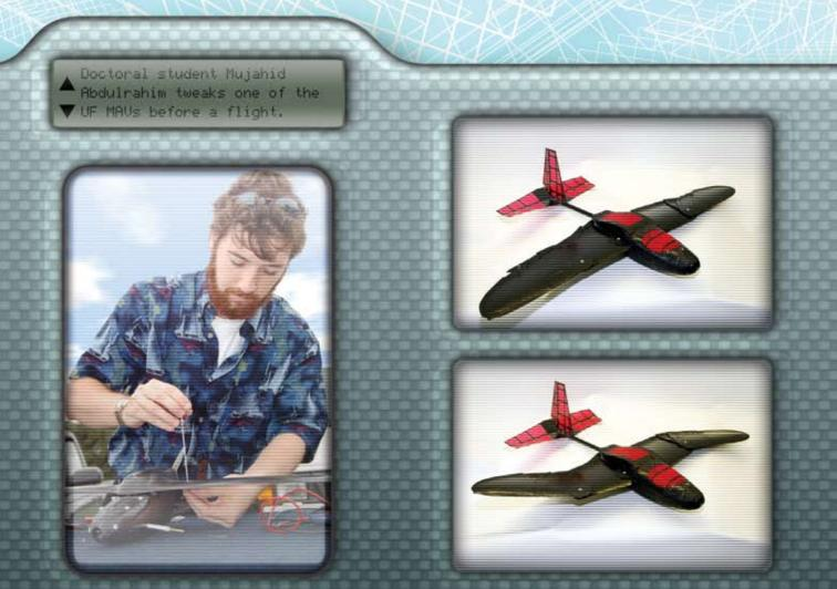
"morph," or change shape, dramatically during flight, transforming the planes' stability and agility. With the wings in the down position, the plane loses stability but becomes highly maneuverable. With the wings in the elbow-straight position, it glides well. And with the wings in the elbow-up position, it's highly controllable and easy to land.
