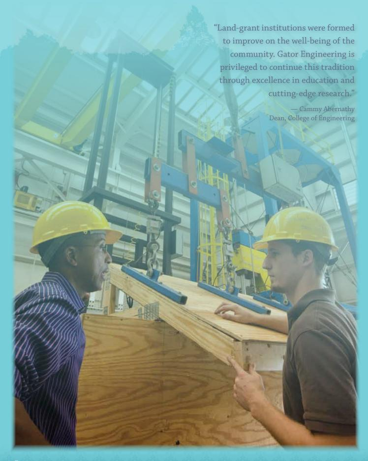
**Engineers say Lessons Learned From Hurricanes can also be applied to Tornadoes**Civil engineer David O. Prevatt, left, and graduate student David Roueche are testing ways to keep roofs attached to structures during storms with strong winds.
